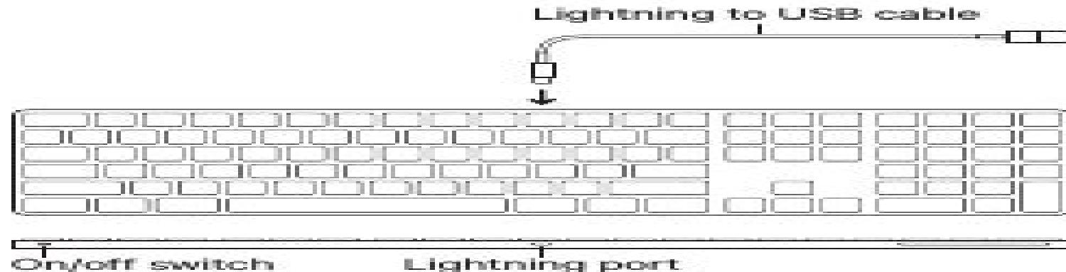
Use the Lightning to USB cable that came with your keyboard. Plug the Lightning end into the Lightning port on your keyboard.
