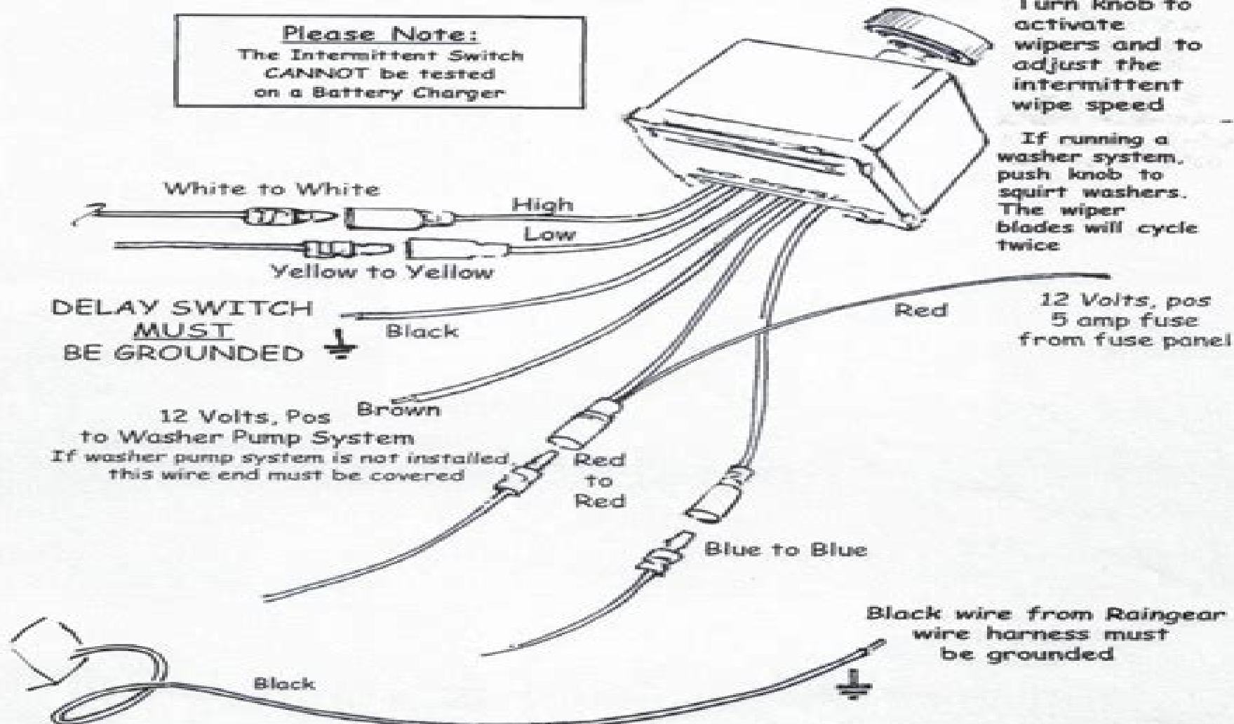
**NOTE:** The colors of the wires from the wiper
