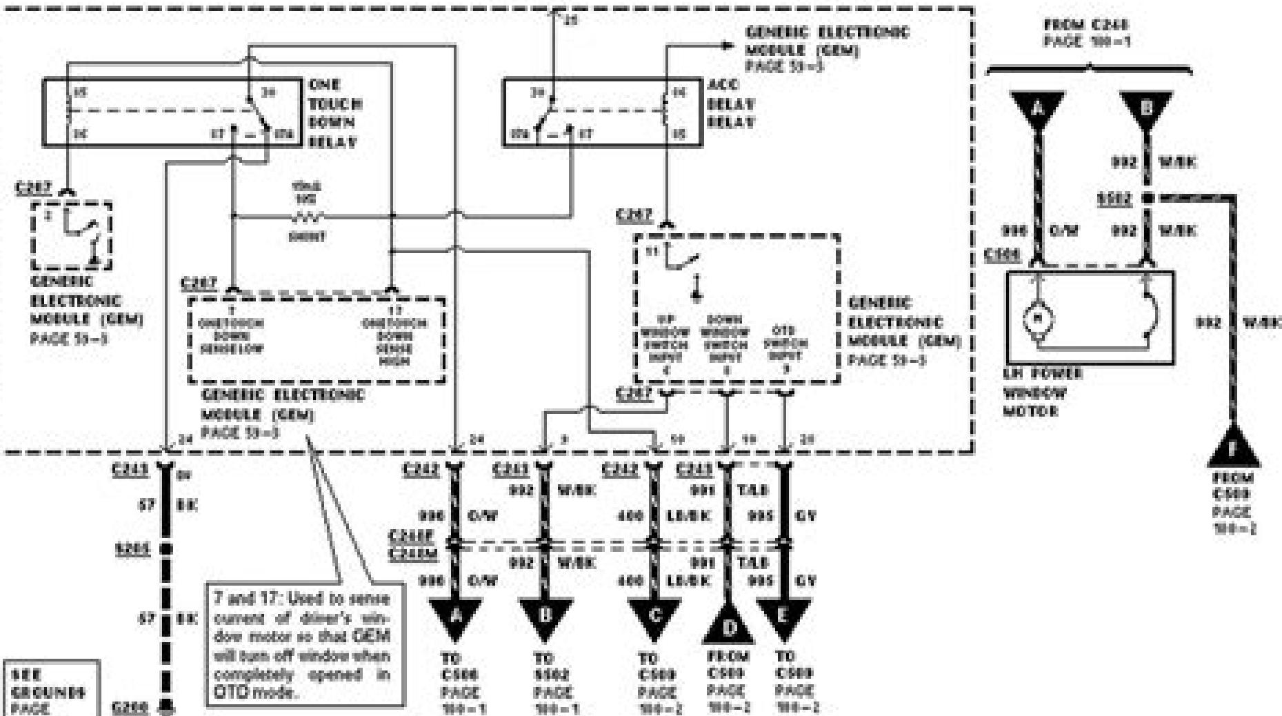
7 and 17: Used to sense current of driver's window motor so that OEM will turn off window when completely opened in GTC mode.
