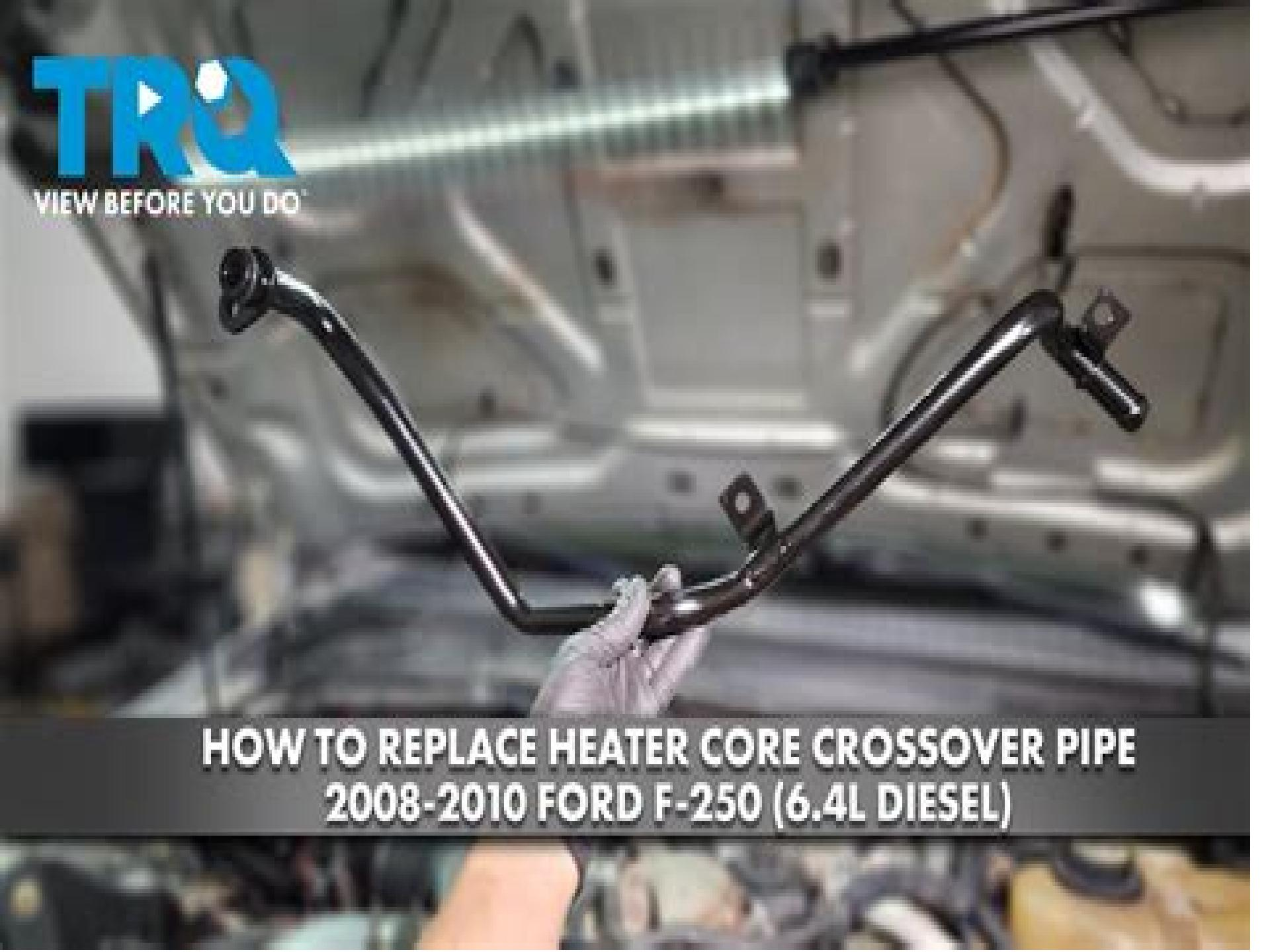
A close-up, slightly blurred photograph of a vehicle's engine compartment. The focus is on a black metal heater core crossover pipe that branches off from a larger pipe. The pipe is secured with clamps and has a flared end. The background is filled with various engine components like hoses and metal brackets.
