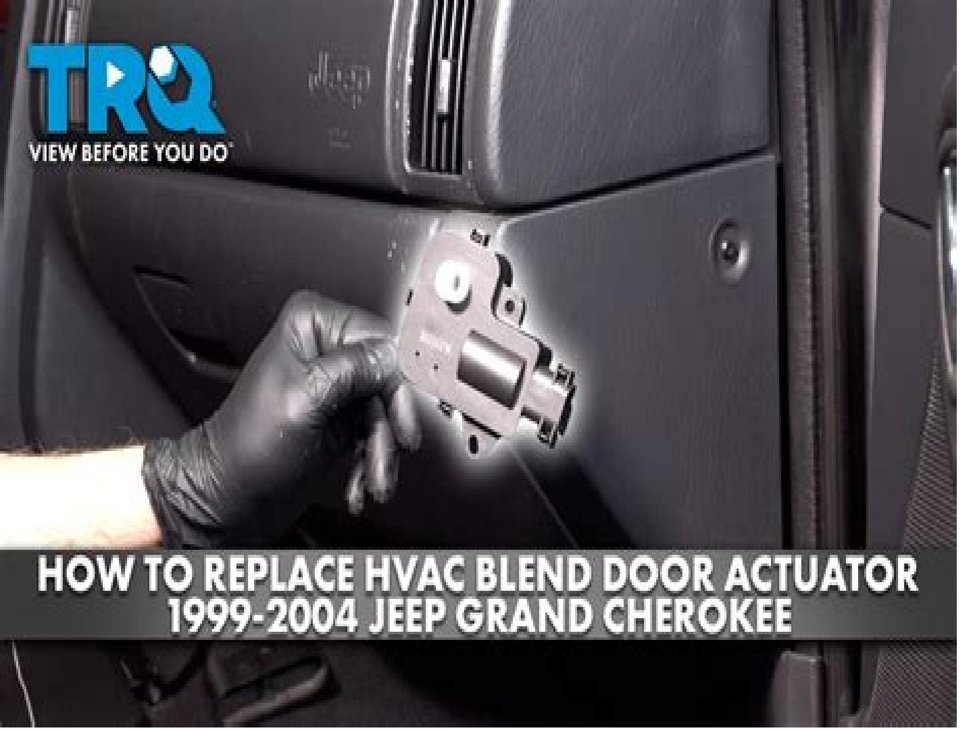
**HOW TO REPLACE HVAC BLEND DOOR ACTUATOR
