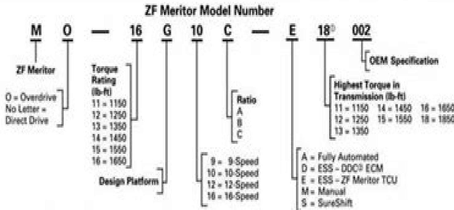
② Progressive torque is an engine feature that requires a Torq-2 transmission. In models not featuring progressive torque, this number will be the same as the torque rating.
