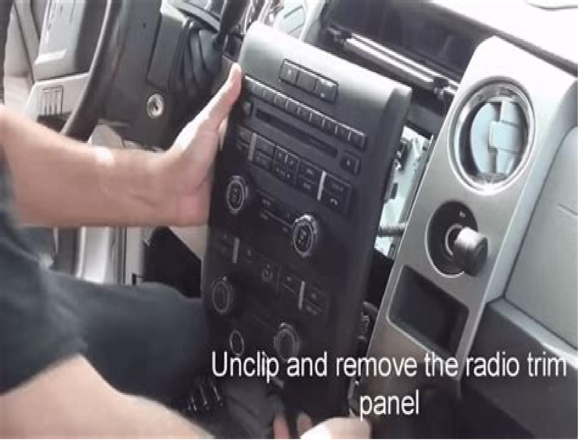
Unclip and remove the radio trim panel
