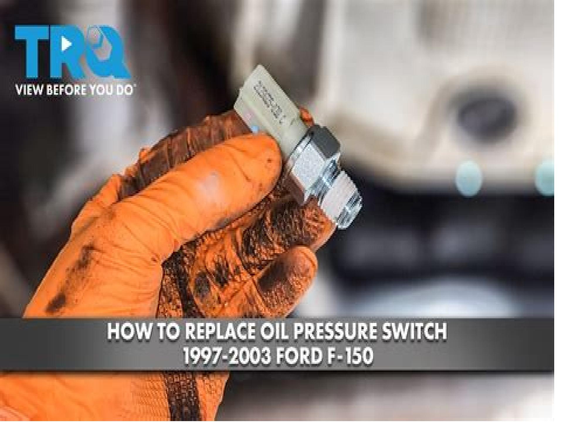
A close-up photograph showing a person's hands wearing orange work gloves. They are working on a mechanical component, specifically an oil pressure switch, which is mounted on a metal pipe. The switch has a blue and silver cylindrical body with a white label that is partially visible. The background is blurred, showing parts of a car's engine and a wrench.
