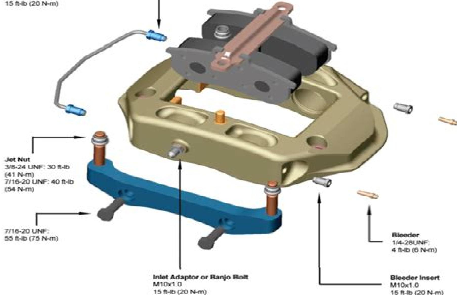
Note: All torque specifications are at ambient temperature
