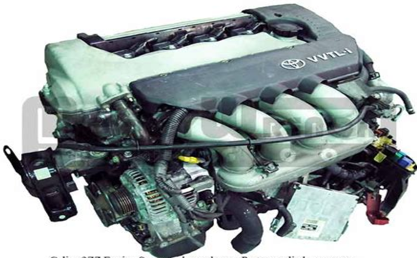
Celica 2ZZ Engine Swap package shown. Parts supplied may vary - check package description for list of items included.
