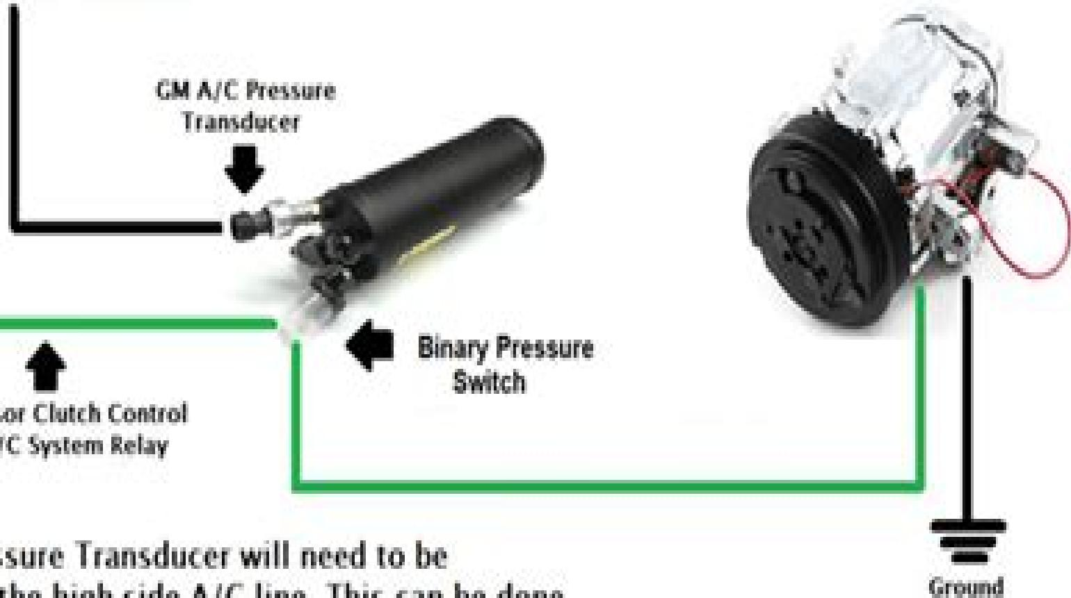
The GM Pressure Transducer will need to be mounted in the high side A/C line. This can be done with the pictured receiver drier, our tee in fitting, or our weld in fitting. This transducer is REQUIRED for the PCM to control fans while the A/C is running. Forcing the fans on with a relay will drastically decrease fan life as the fans will be on even at cruising speeds.
