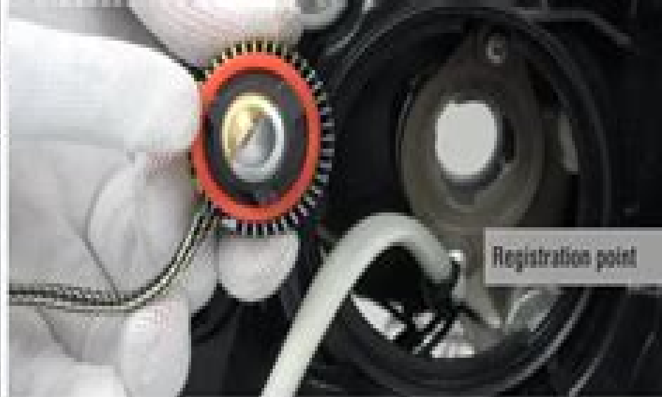
② Insert the LED bulbs into the housing.
