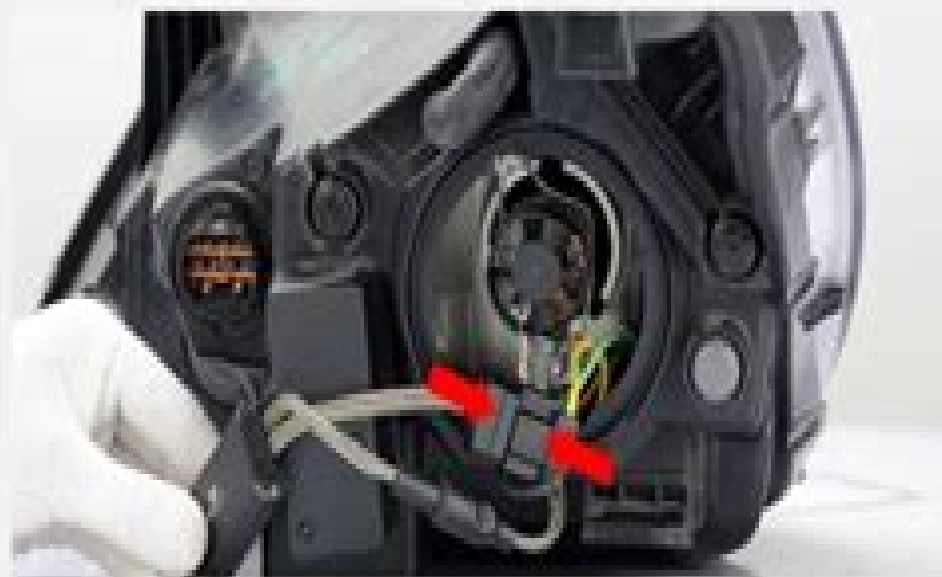
④ Connect to the headlights power.
