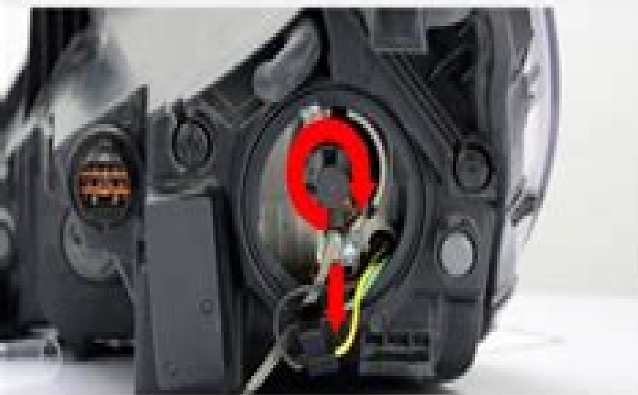
③ Rotate clockwise to lock, with wire down at 6 o'clock.
