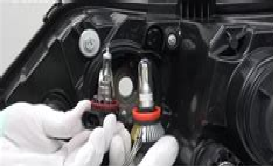
① Take out the original halogen bulbs.
