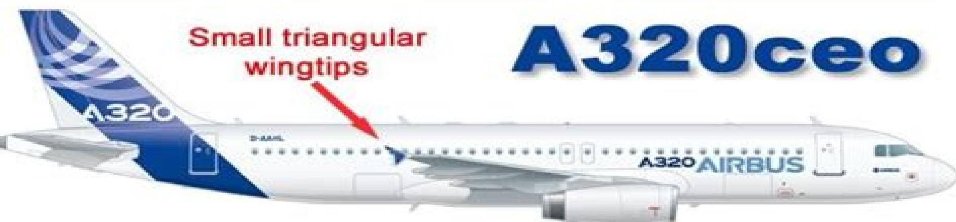
Smaller engine, with no trailing extensions at rear
