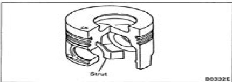
The pistons for the 6D16 engine have an internal strut to reduce piston slap noise.
