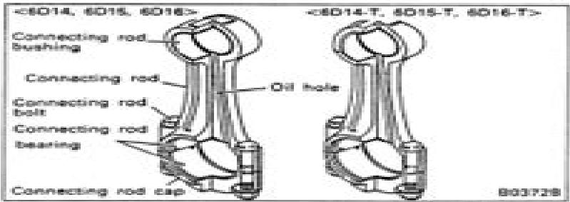
The connecting rod is a die-forged part with I-section. It has a lead bronze bushing press fitted at the small end and a split type plain bearing fitted at the big end of the connecting rod.
