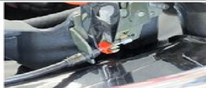
apply and tighten the nuts for fastening the saddle opening device's bracket.
