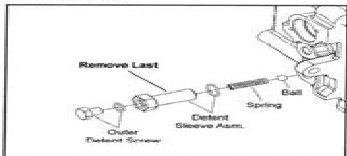
**NOTE: DO NOT** remove the detent sleeve assembly before removing the outer detent screw. Removing the detent sleeve first will allow the detent ball and spring to fall into the shift housing.
