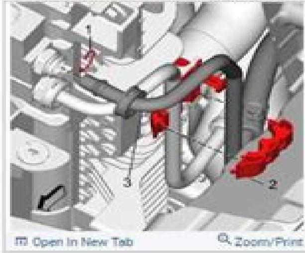
5. Transmission Fluid Cooler Inlet Pipe Clip (1) - Remove — Transmission Fluid Cooler Hose/Pipe Quick-Connect Fitting Disconnection and Connection
