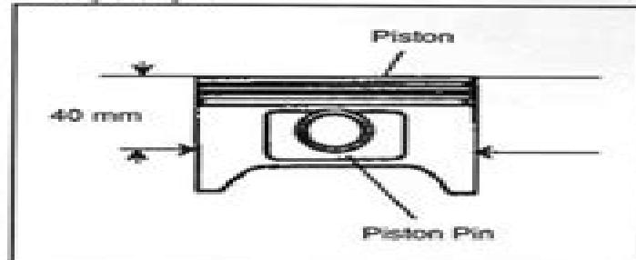
2. Subtract this measurement from the maximum cylinder measurement obtained in Step 5 above.
