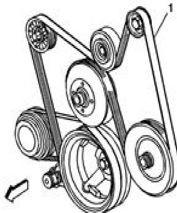
Fig. 2: View Of Drive Belt (4.8L, 5.3L, and 6.0L Engines)
