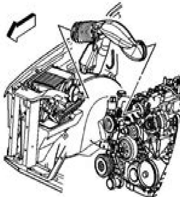
Fig. 1: View Of Air Cleaner Outlet Duct
