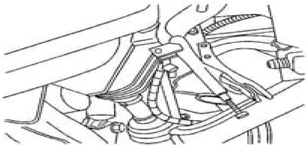
Fig. 4: Installing The Dial Indicator Between The Pitman Arm And Relay Rod
