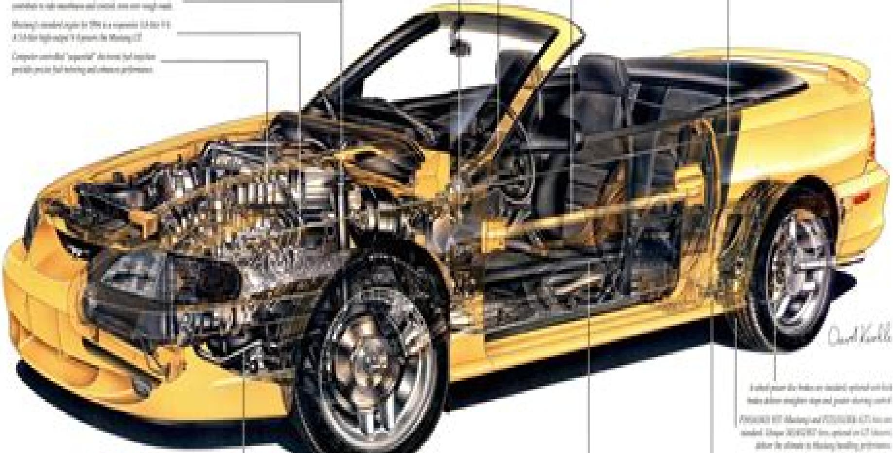
Front and rear disc brakes with optional air suspension, front and rear, contribute to smooth ride and greater steering control.
