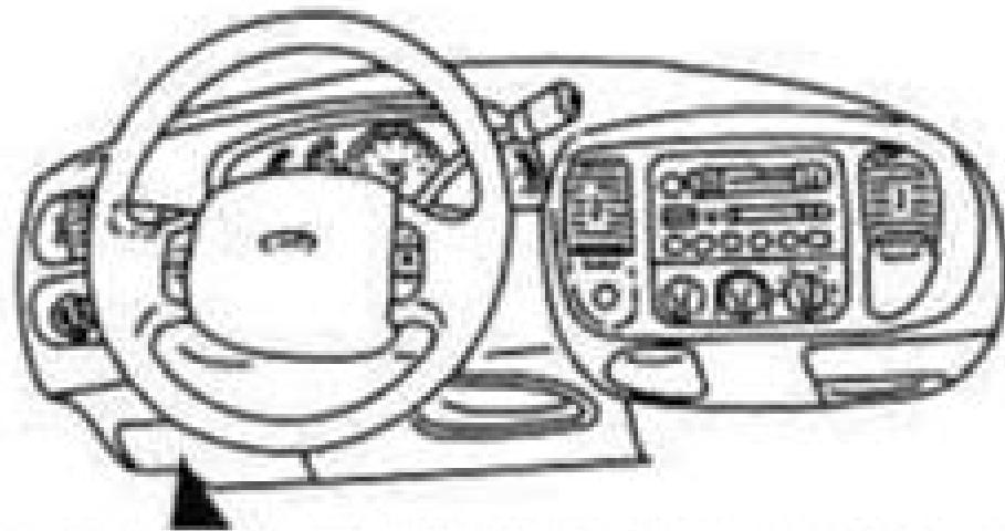
The fuse panel is located below and to the left of the steering wheel by the brake pedal. Remove the panel cover to access the fuses.
