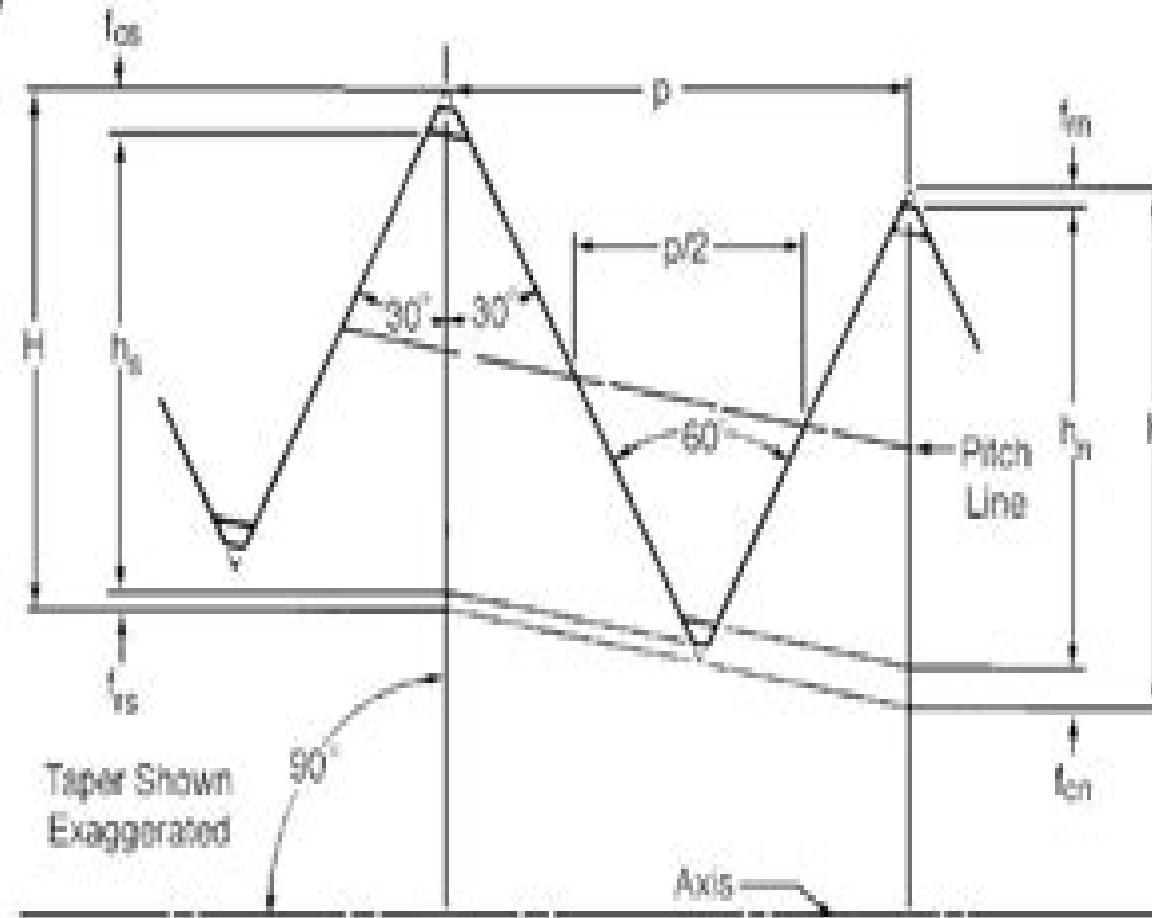
Taper =  $\frac{3}{4}$  in. per ft or 0.0625 in. per in. on Diameter
