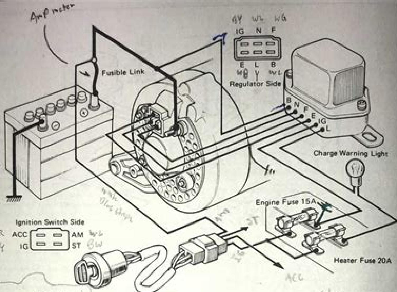
Fig. 11.2. Alternator connections - charge warning light types
