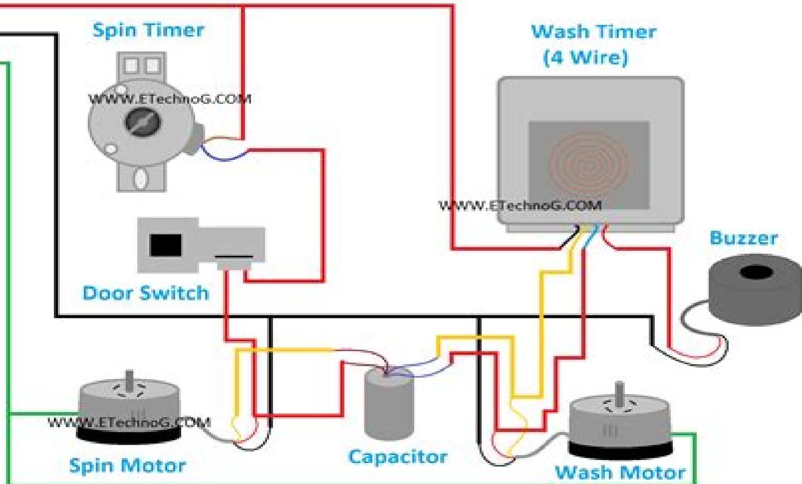
**Washing Machine Wiring and Connection Diagram**
