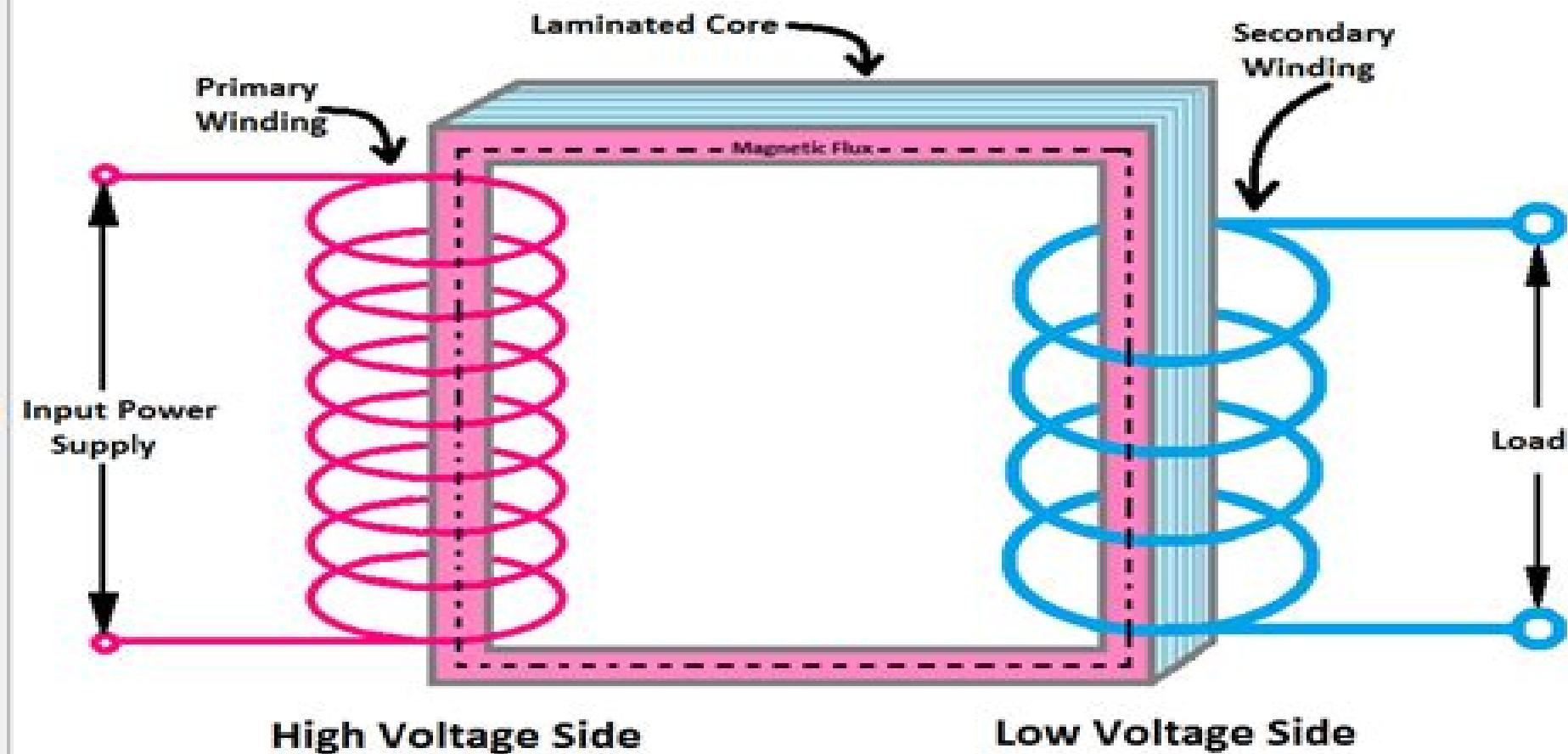
**Step Down Transformer Diagram**
