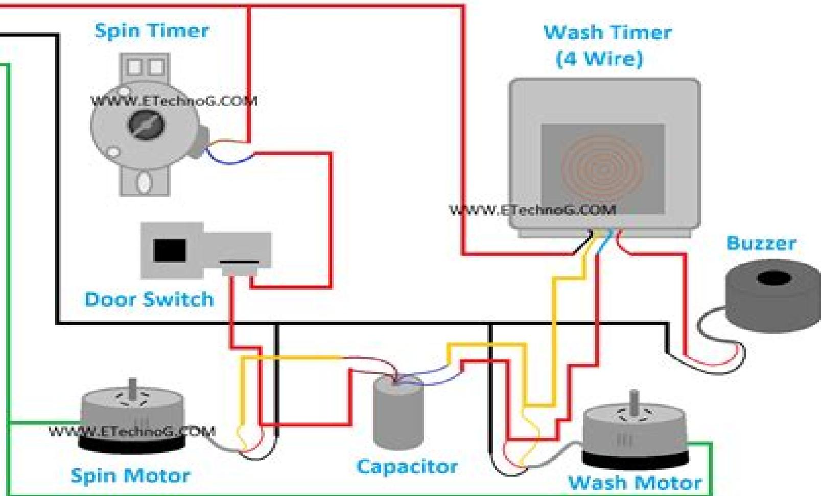
**Washing Machine Wiring and Connection Diagram**
