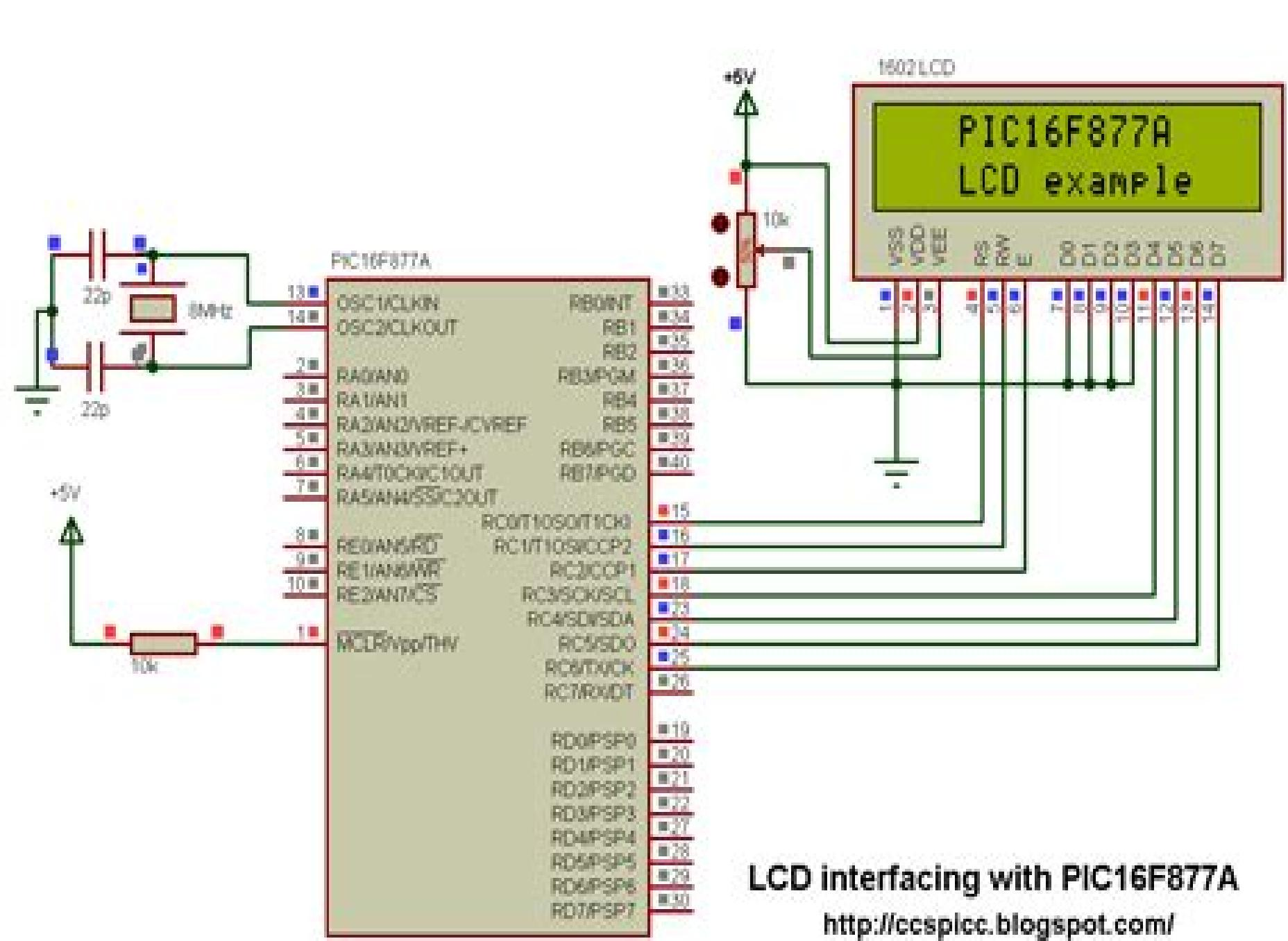
**LCD interfacing with PIC16F877A**
