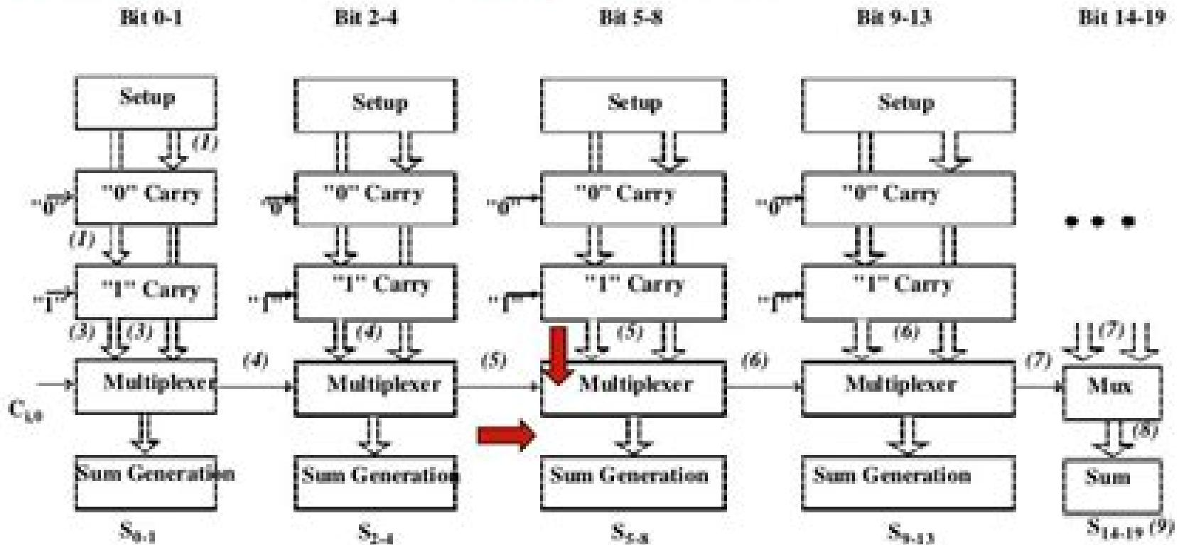
$$t_{add} = t_{setup} + P \cdot t_{carry} + (\sqrt{2N})t_{mux} + t_{sum}$$
