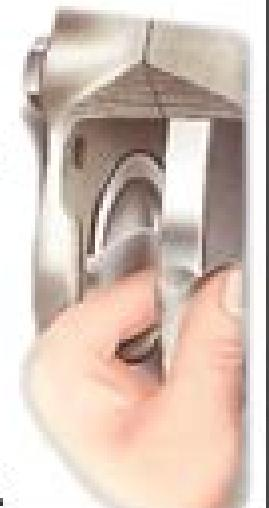
Pull out the pad retaining clip with pliers.
