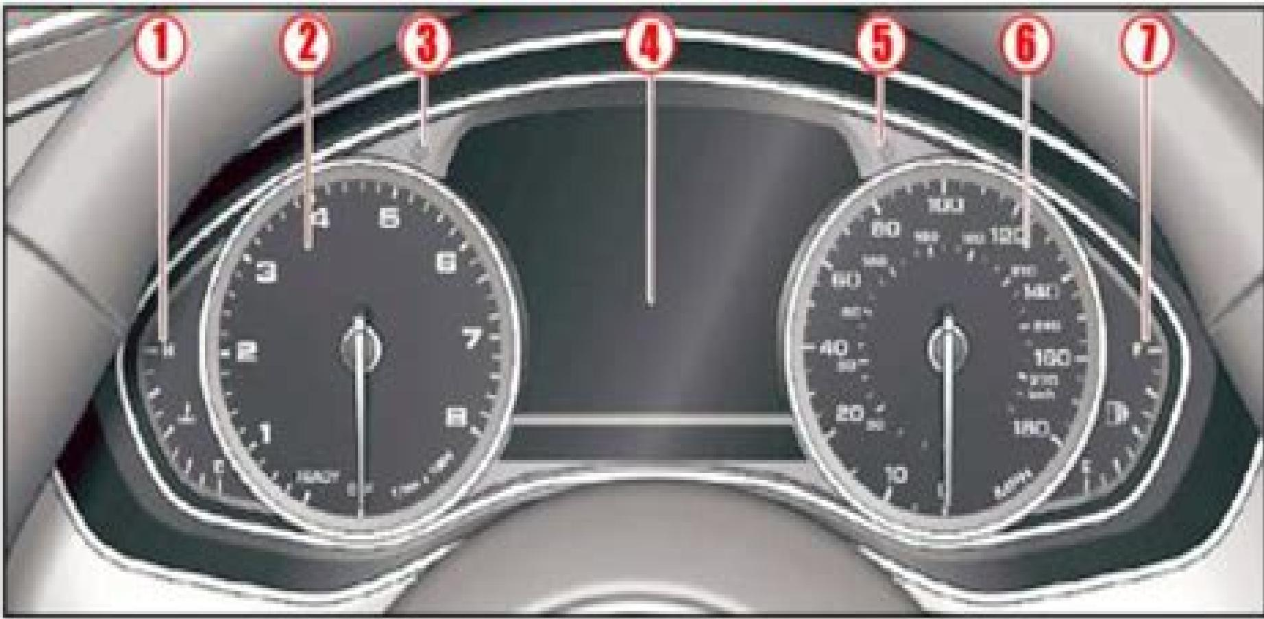
1. Engine Coolant Temperature Gauge;
