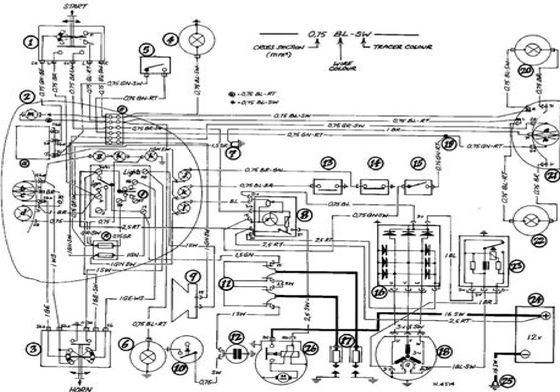
Wiring diagram - /5 models
