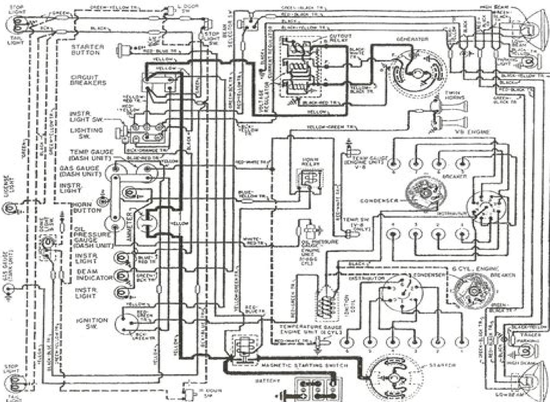
1951-1952 FORD TRUCKS LIGHT DUTY F-1, F-2, F-3 & HEAVY DUTY F-4, F-5 & F-6 WIRING DIAGRAM
