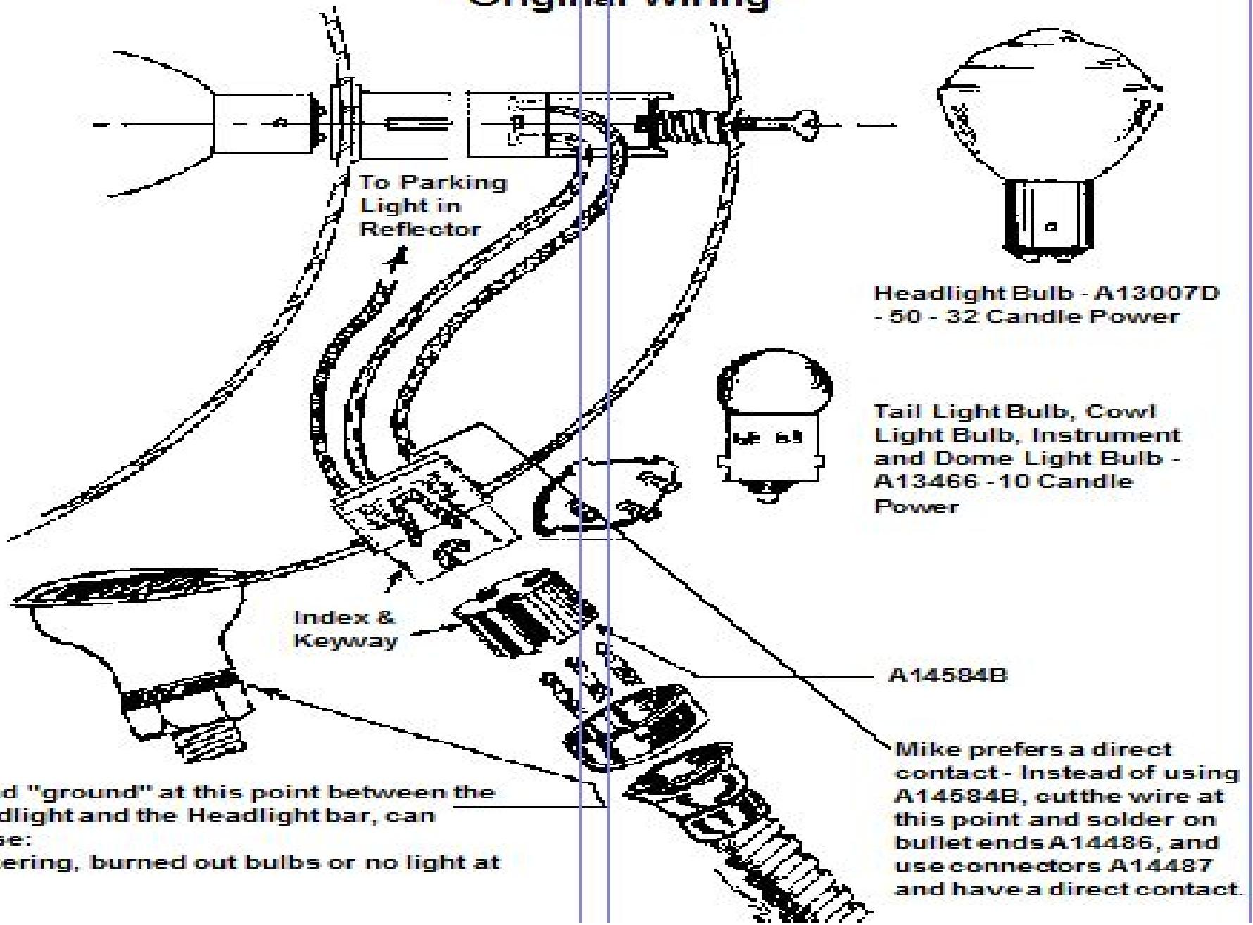
A bad "ground" at this point between the Headlight and the Headlight bar, can cause:
