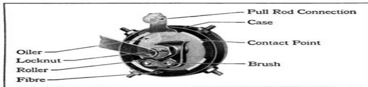
connected with a coil unit, an electrical circuit is passed through the entire system of primary wires. This circuit is only momentary, however, as the roller passes over the contact point very rapidly and sets up the circuit in each unit as the roller touches the contact point connected with that unit. The commutator should be kept clean and well oiled at all times.
