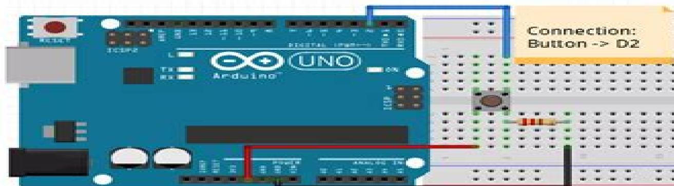
Connect three wires to the board. The first two, red and black, connect to the two long vertical rows on the side of the breadboard to provide access to the 5 volt supply and ground. The third wire goes from digital pin 2 to one leg of the pushbutton. That same leg of the button connects through a pull-down resistor (here 10K ohm) to ground. The other
