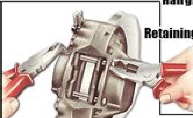
Pull out the pad retaining clip with pliers.
