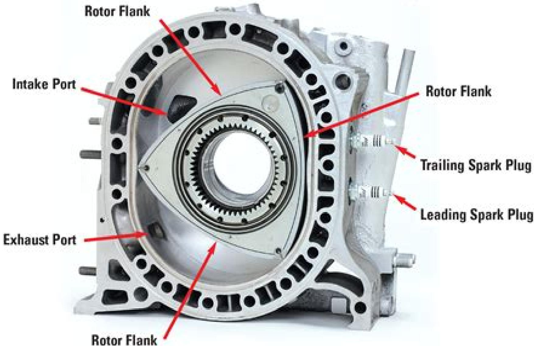
Each rotor flank encloses a working chamber in the rotor housing.
