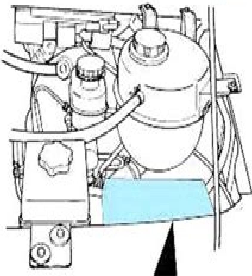
The power distribution box is located in the engine compartment. The power distribution box contains high-current fuses that protect your vehicle's main electrical systems from overloads.
