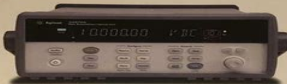
Agilent 34970A Data Acquisition / Switch Unit
