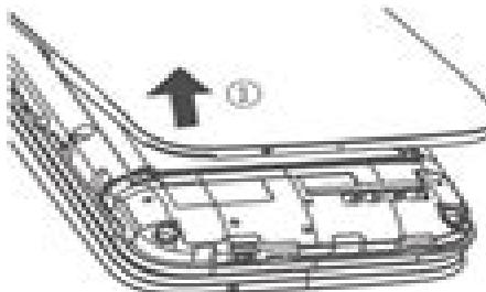
① Removing or installing the back cover.
