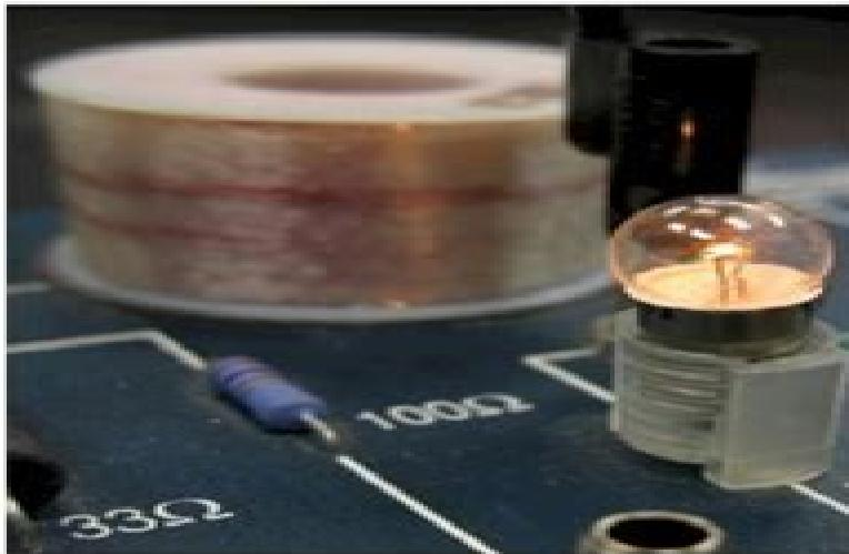
This lit bulb is part of an AC circuit. The coil of wire in the background would have no effect on a DC circuit, but is a key component of an AC circuit. It is called an "inductor."
