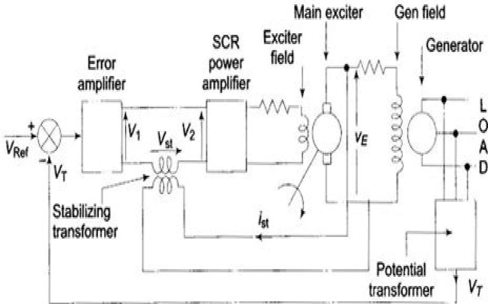
Fig. 8.20 Schematic diagram of alternator voltage regulator scheme
