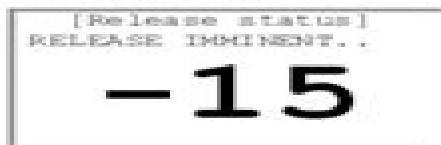
The display shows a countdown timer with the amount of time remaining before the extinguishant is released.
