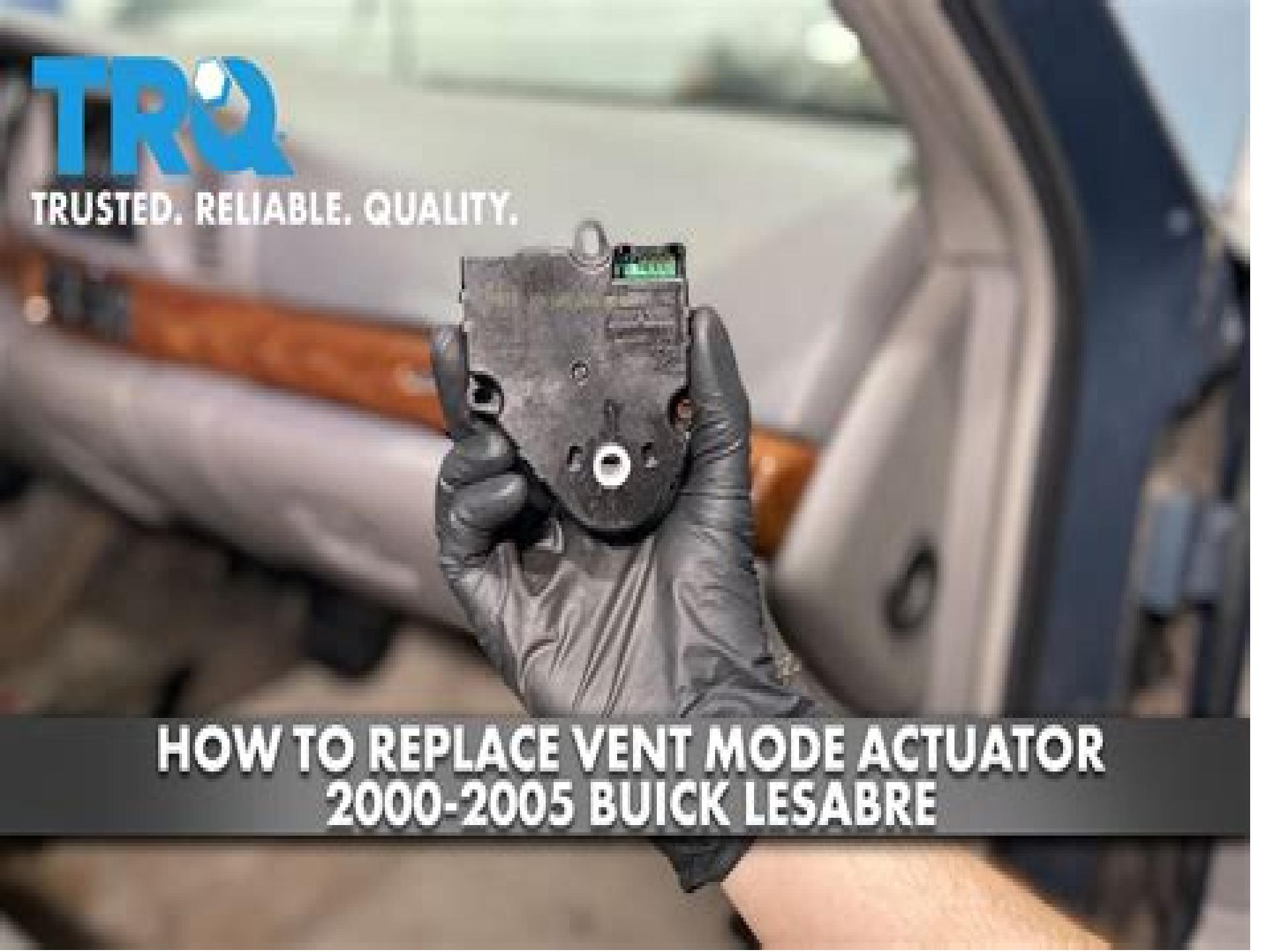
**HOW TO REPLACE VENT MODE ACTUATOR
