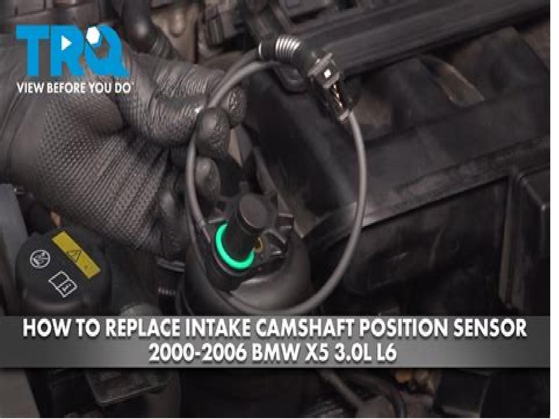
HOW TO REPLACE INTAKE CAMSHAFT POSITION SENSOR
