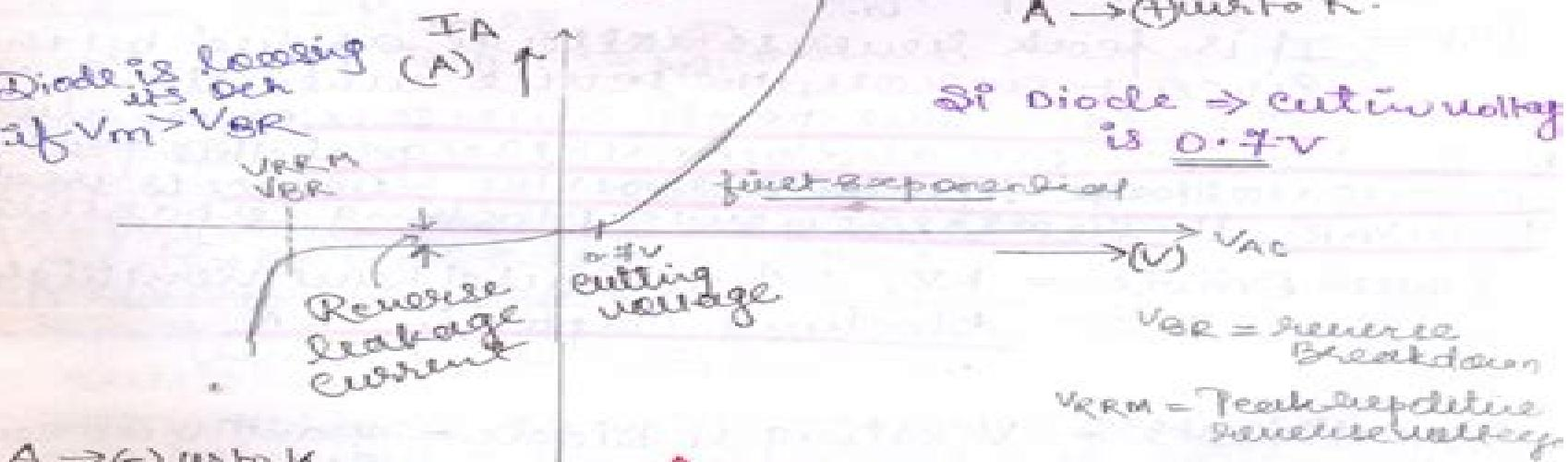
Diode  $\rightarrow$  cut-in voltage is 0.7V
