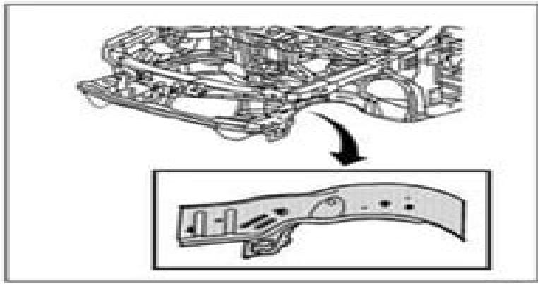
7. Remove the outer rail from the vehicle.
