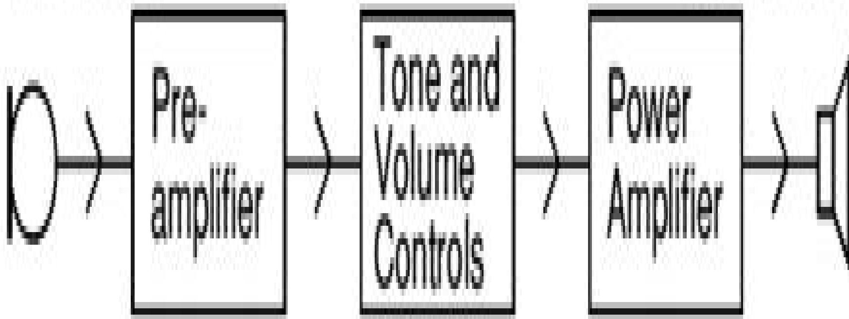
Block Diagram of an Audio Amplifier System
