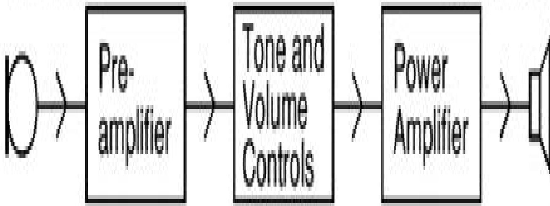
Block Diagram of an Audio Amplifier System
