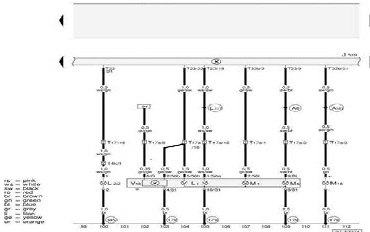
JS19 - Vehicle Electrical System Control Module
